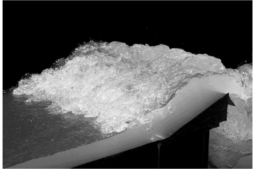
Hydraulic jump modelled after Froude
